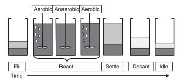
Fig. 1. Typical sequencing batch reactor operation.
