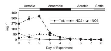
Fig. 2. Concentration of ammonia (TAN), nitrate (NO3) and nitrite (NO2) in wastewater sludge during operation of SBR for 8 days. Results are mean values for four reactors  $\pm$  SD.
